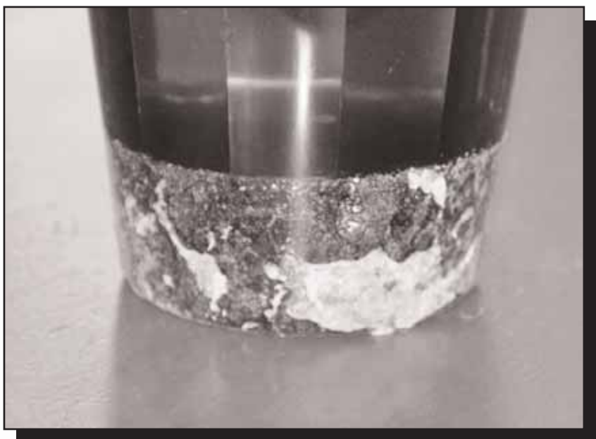
Example of a created waterline using talcum powder
