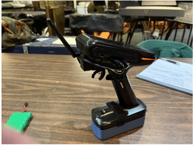
The blue at the base is the new battery pack
